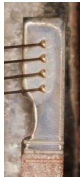
Figure 29 – Plated Ag Visible in the Area Around the Stitch Bonds, Cu only Visible at Edges
