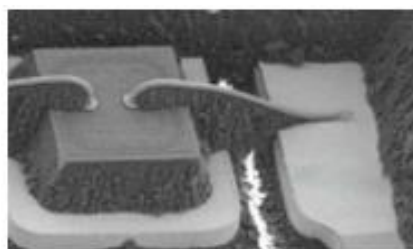
Figure 25 – Laser Ablation Damage
